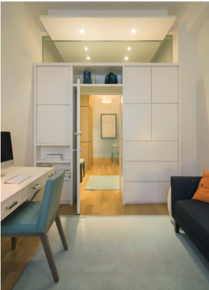
A window built into the partition lets light in and creates a feeling of openness within the small space. Photo by Bjorg Magnea
